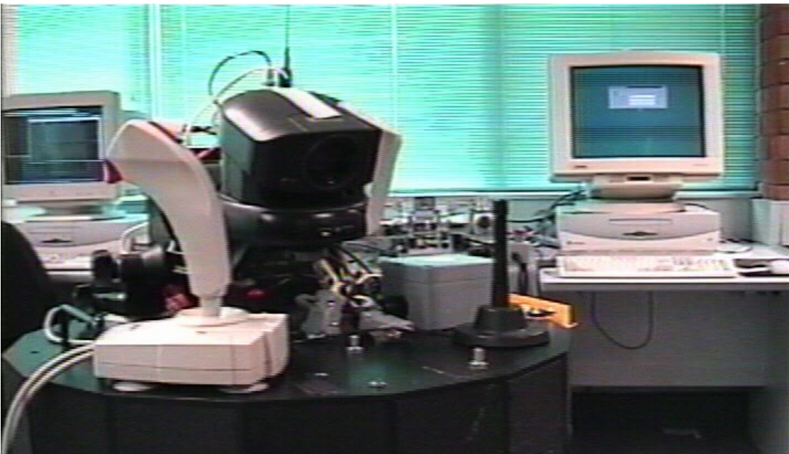
Figure 6.2: Uncalibrated camera mounted on the Nomad 200
