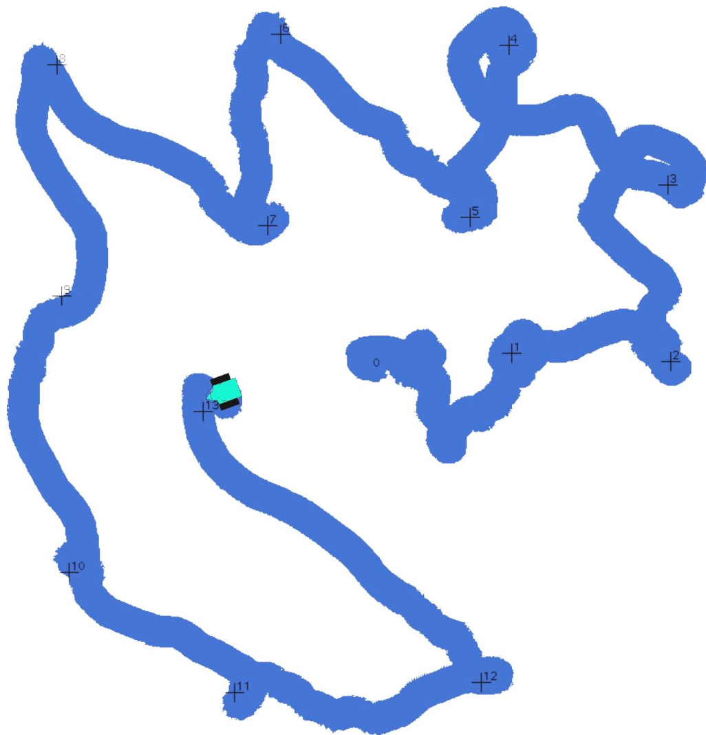
Figure 3.11: Appearance of the simulation for one run. The boat begins at the point marked 0. Targets are marked with a + symbol and target number. The boat gradually learnt to control its motion and move more directly to targets.
