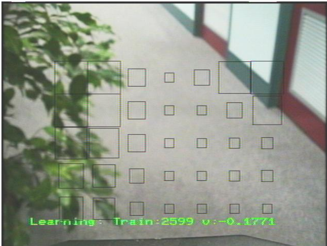
Figure 6.4: The robot's view during the wandering behaviour. Small squares indicate a good match with the carpet template; accordingly, large squares represent detected obstacles.
