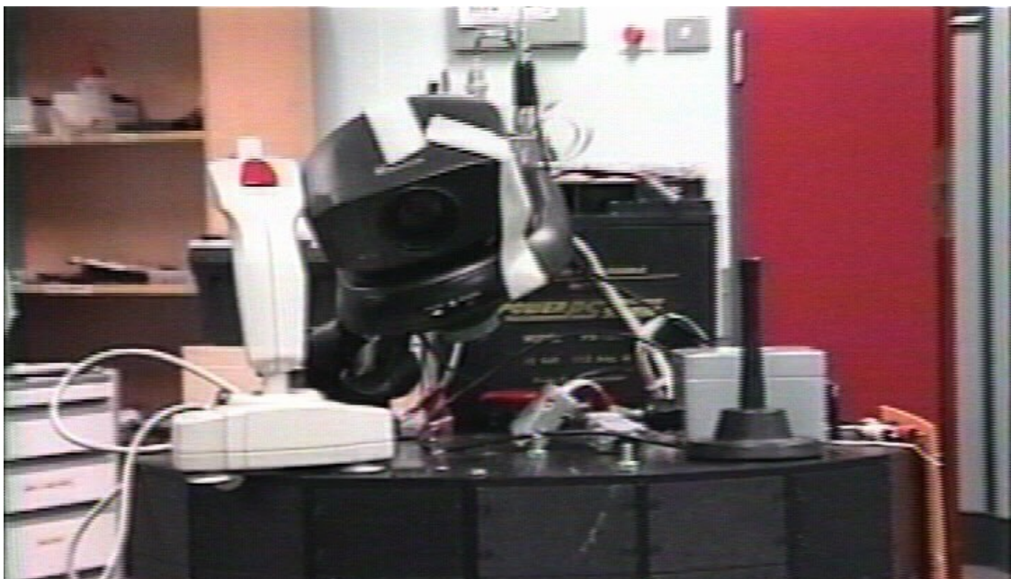
Figure 6.14: The camera is misaligned, pointing in a different direction from the translation axis
